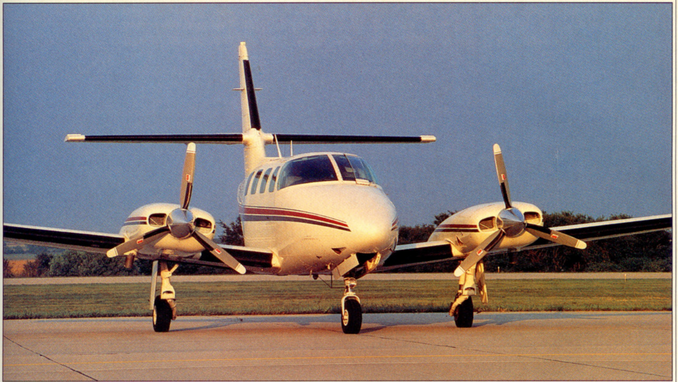
A light twin with heavy-twin aspirations (above). The distinctive cruciform tail is one of the Crusader's identifying features. The horizontal stabilizer rides up and out of wing wake and prop wash.
